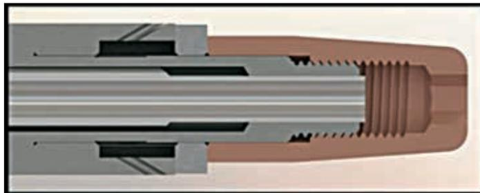
Figure 1: Indirect Water Cooled (water transfer)
