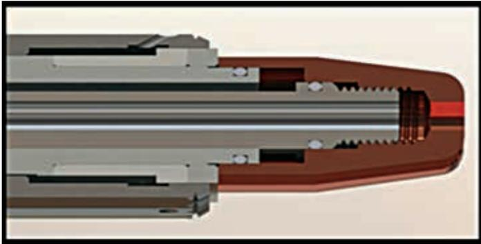
Figure 3: Direct Water Cooled (spring loaded sleeve)
