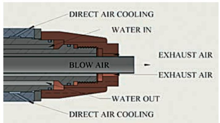
Figure 5: Air / Water flow (Recirculating air)
